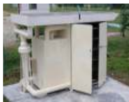
Fig. 19: Photograph of solar assisted heat pump dryer with multifunctional solar collector
