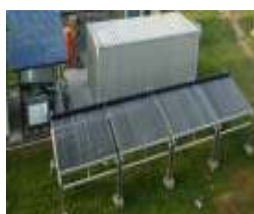
Fig. 27: Photograph of solar desiccant dryer system
