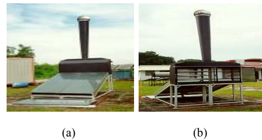
Fig. 2: Photograph of natural convection solar dryer; (a) view from solar collector and (b) view from drying chamber
