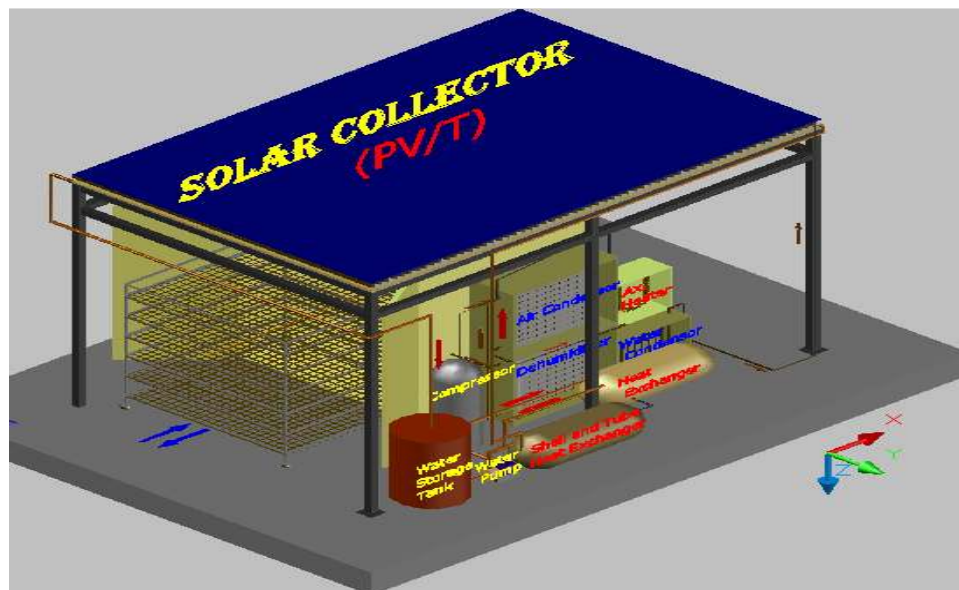
Fig. 21: Configuration of solar assisted heat pump dryer with PV/T water based collector
