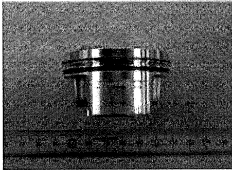
A2618 Heat-resistant Al alloy Cylinder bore : Ni-P plating
