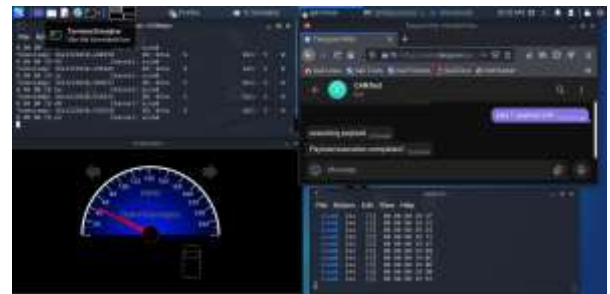
Fig. 4 Result on IC Simulator speedometer after replay attack
