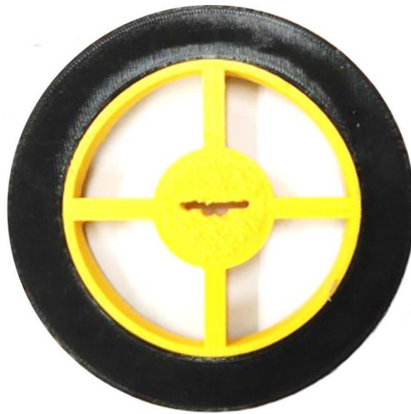
Figure 2. The fabricated PEC NDT probe with a slot at the centre where the TMR PCB will be inserted in order to place the sensor as centred as possible.
