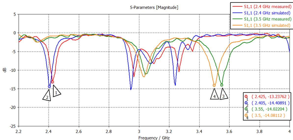
**Figure 4.** Simulated and measured S11 of 2.4 GHz and 3.5 GHz patch antenna
