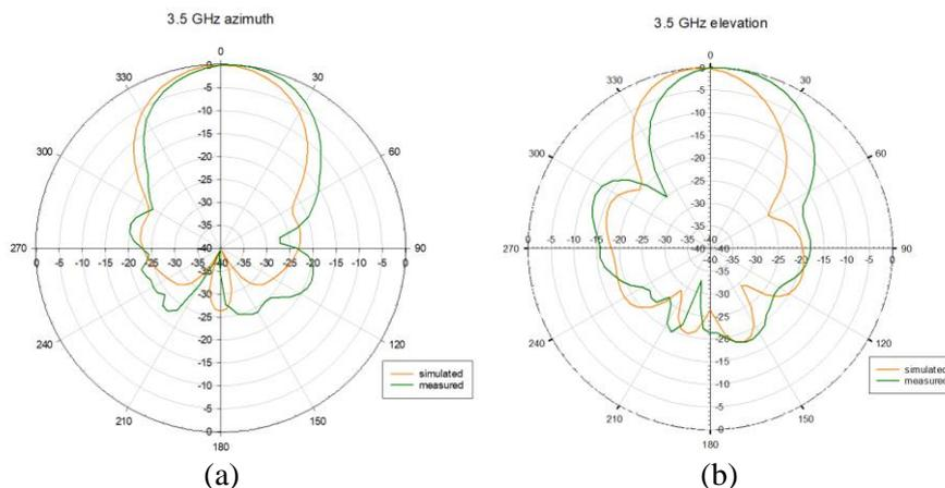
**Figure 6.** Simulated and measured (a) H-plane and (b) E-plane pattern at 3.5 GHz
