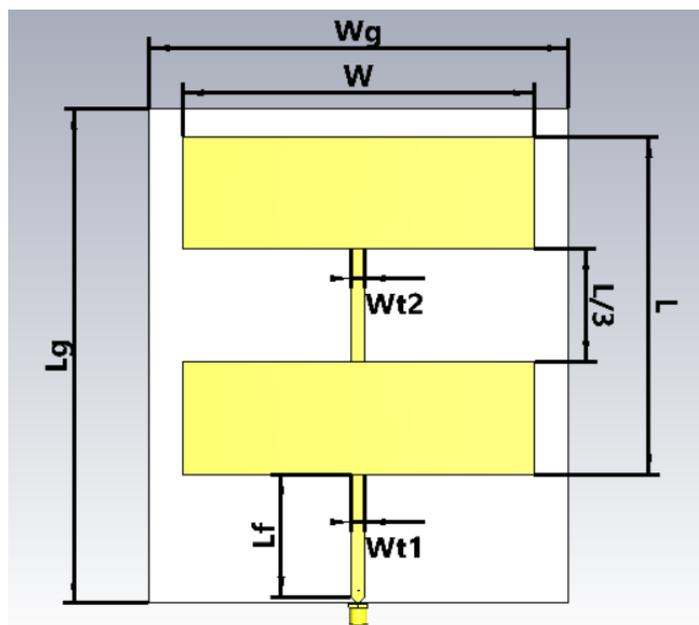
**Figure 1.** Patch antenna configuration (Top view)
