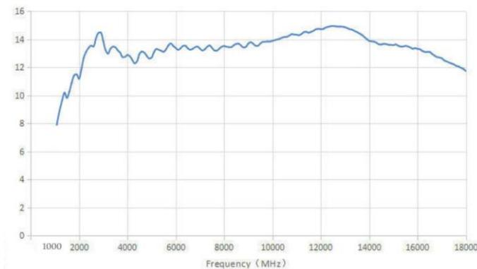
**Figure 7.** The gain of standard horn antenna [10]
