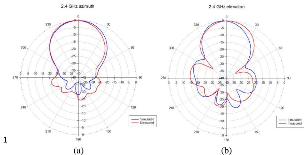
**Figure 5.** Simulated and measured (a) H-plane and (b) E-plane pattern at 2.4 GHz
