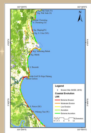
Figure 3: Digital Shoreline Analysis System output using Landsat 8.
