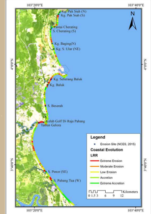
Figure 2: Digital Shoreline Analysis System output using Sentinel-2
