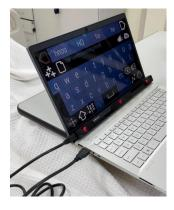
**Image 1**: This image illustrates Ms A operating the keyboard using an electronic eye tracker device attached at the bottom of the laptop screen.
