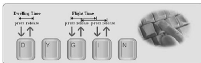
Fig. 5. Dwell time and flight time of keystroke biometrics [9].
