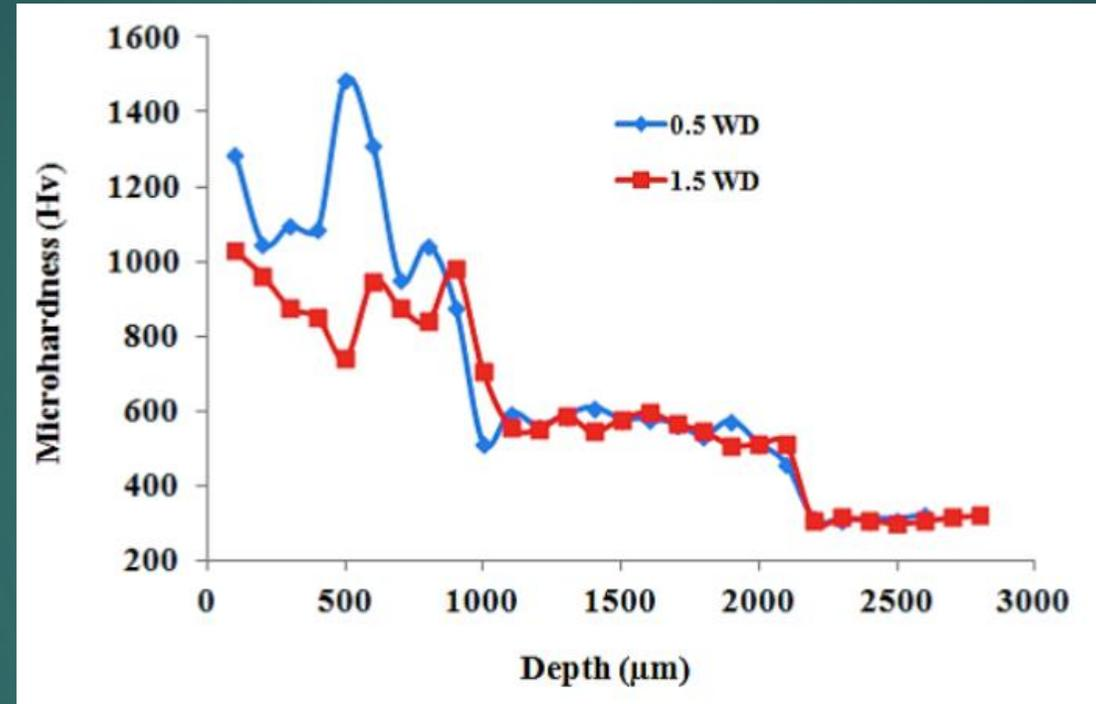
Overwhelmed reprecipitation near the arc source gave hardness between 1000HV to 1500 HV with 0.5 mm working distance
