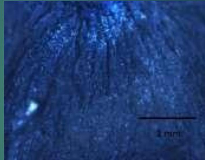
Less viscous from stirring action in the melt resulted ripples on the solidified surface.
