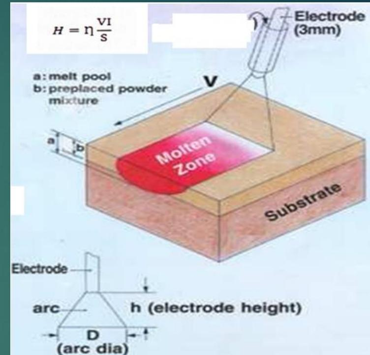
Illustration describing the TIG melting of preplaced particulates on substrate
