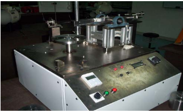
Figure 3 Photograph of the wear and friction test apparatus
