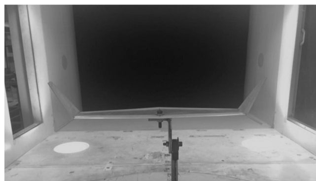
Wind tunnel test of a wing model in the IUM low speed wind tunnel
