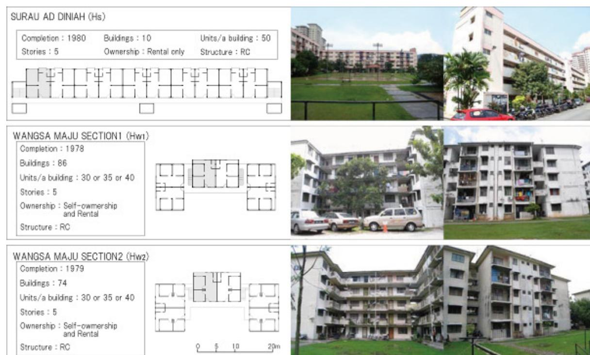
Fig.2 Surveyed apartments of a housing complex building plan and basic information
