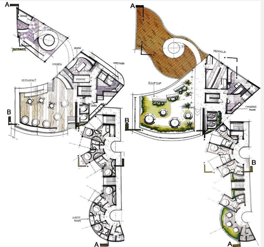
Figure 10: First and second floor plan ( Scale 1:100)
