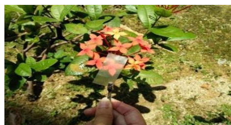
Figure 1: Translucent chitin thin film: treated with 6% NaClO for 4 h at 28°C
