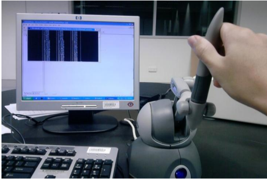
Fig. 2. Touching the virtual object by using PHANTOM Desktop
