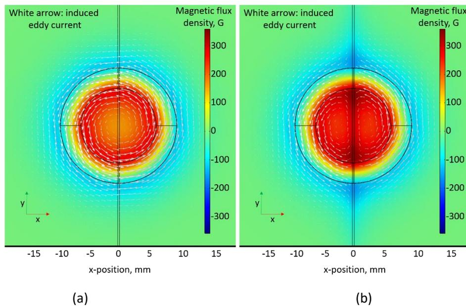
Figure 8 Top view of magnetic flux density for (a) flawless sample and (b) sample with 90° crack
