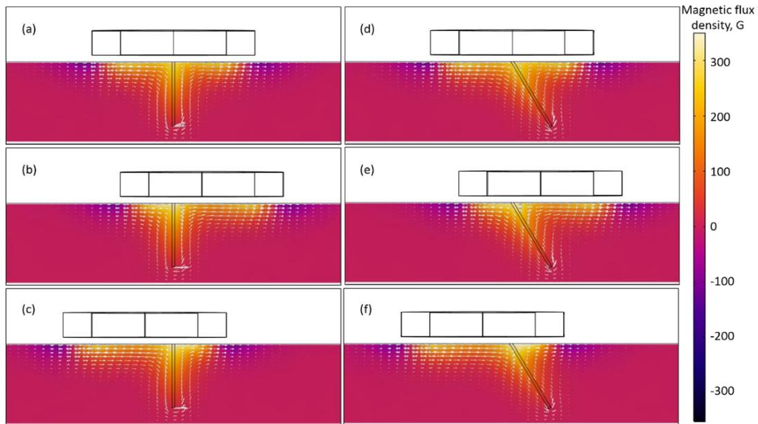
Figure 9 Magnetic field distribution of crack of (a)  $90^\circ$  at 0 mm, (b)  $90^\circ$  at 3.5 mm, (c)  $90^\circ$  at -3.5 mm, (d)  $60^\circ$  at 0 mm, (e)  $60^\circ$  at 3.5 mm and (f)  $60^\circ$  at -3.5 mm
