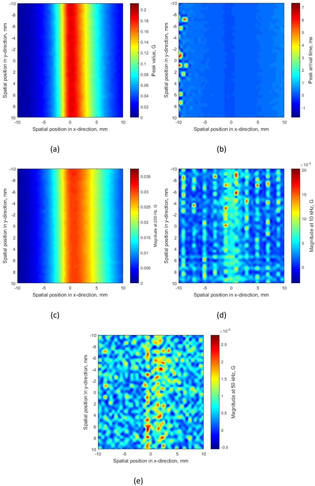
Figure 7 C-scan images constructed using (a) peak value, (b) peak arrival time, (c) magnitude at 200 Hz, (d) magnitude at 10 kHz, (e) magnitude at 50 kHz
