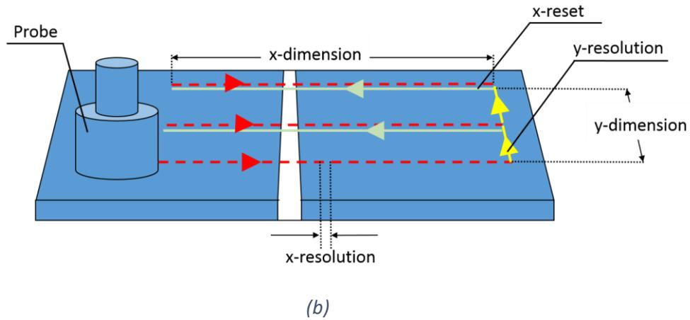
Figure 5 (a) The state machine of the LabVIEW graphical codes and (b) illustration of the scanning flow
