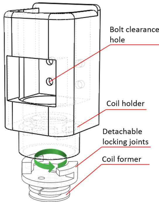
Figure 4 (Geometrical design of the coil former and the coil holder)
