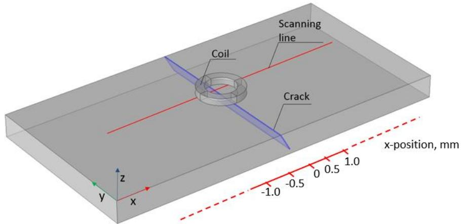
Figure 1 Geometry of the constructed FEM using COMSOL Multiphysics. Crack was configured as a geometry itself, instead of a slot elongating across the test piece width.
