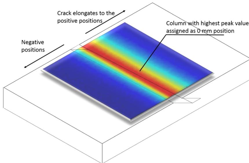
Figure 6 Spatial positioning based on the highest peak value in one of the rows of the image
