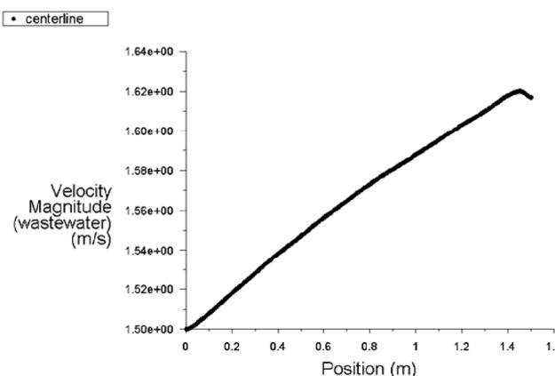
Fig. 4. development of the waste water velocity profile at the center line of the pipe
