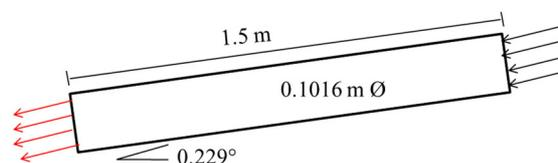
Fig. 1. Description of the simulated pipe
