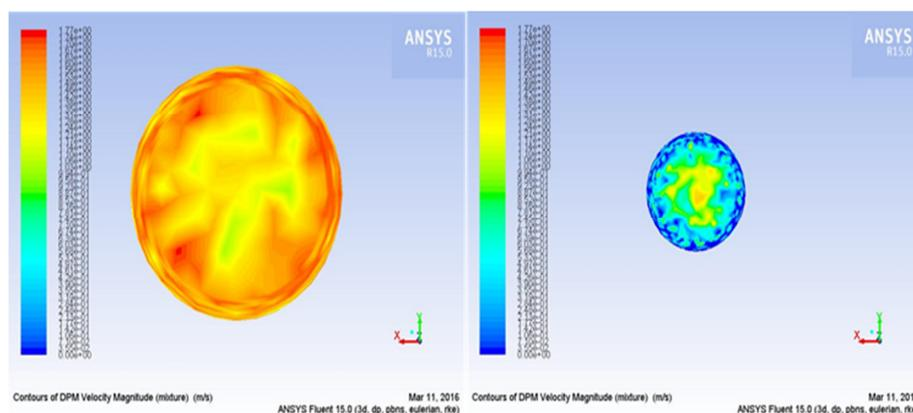
Fig. 3. Velocity contours of FOG particles at the inlet (left) and outlet (right)
