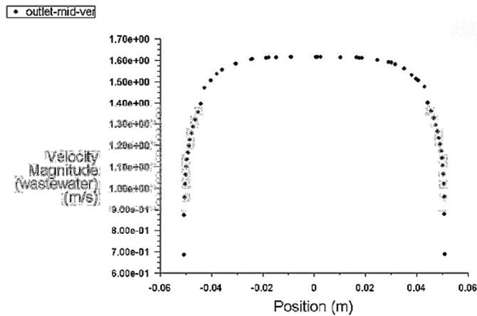
**Fig. 5.** Wastewater velocity distribution at the outlet horizontal line
