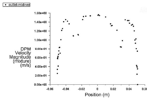
**Fig. 6.** FOG particles velocity at the outlet center line
