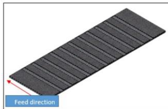
Figure 4 Distance Travelled of carbide cutting Tool for Machining CFRP
