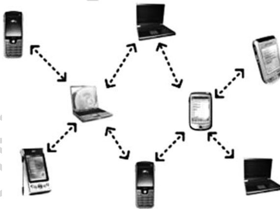
Fig. 4.1. An Example of Mobile Ad Hoc Network (MANET)
