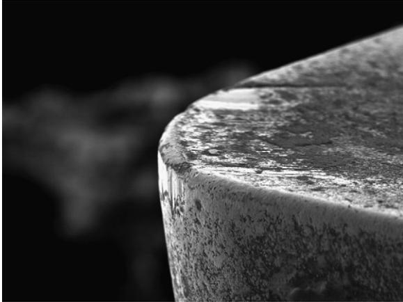
**Fig. 8 – Flank wear after 3 min of machining with cryogenic coolant ( $v = 200$  m/min,  $f = 0.1$  mm/rev and  $t = 0.5$  mm).**
