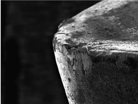
**Fig. 9 – Flank wear after 20 min of machining with conventional coolant ( $v = 100$  m/min,  $f = 0.05$  mm/rev and  $t = 0.5$  mm).**
