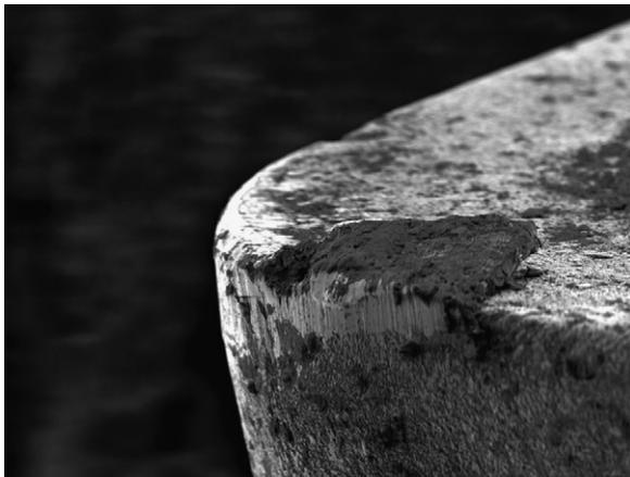
**Fig. 5 – Flank wear after 2 min of machining with conventional coolant ( $v = 250$  m/min,  $f = 0.1$  mm/rev and  $t = 1$  mm).**
