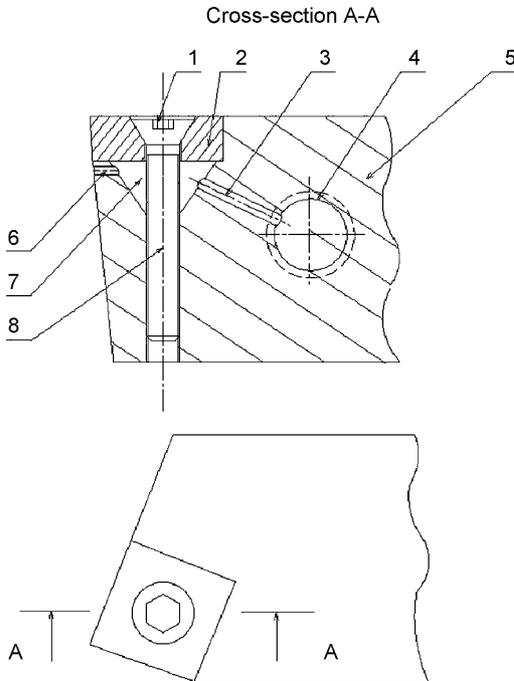
Fig. 1 – Details of the tool for cryogenic cooling.
