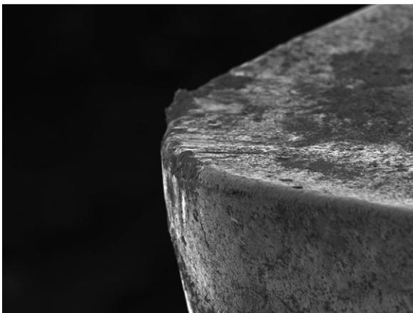
**Fig. 10 – Flank wear after 20 min of machining with cryogenic coolant ( $v = 100$  m/min,  $f = 0.05$  mm/rev and  $t = 0.5$  mm).**
