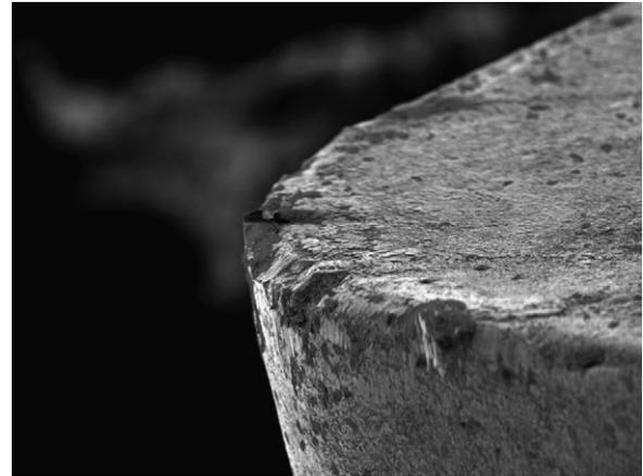
**Fig. 6 – Flank wear after 2 min of machining with cryogenic coolant ( $v = 250$  m/min,  $f = 0.1$  mm/rev and  $t = 1$  mm).**
