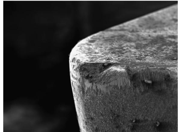
**Fig. 7 – Flank wear after 3 min of machining with conventional coolant ( $v = 200$  m/min,  $f = 0.1$  mm/rev and  $t = 0.5$  mm).**
