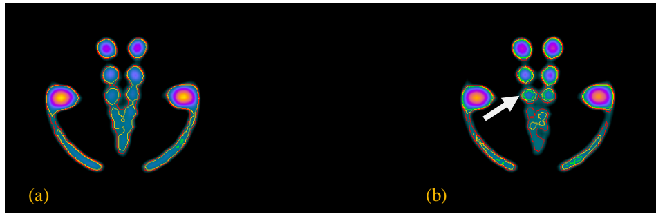
Fig. 4 (a) and (b) show the transverse images hot regions (a) without and (b) with material filter
