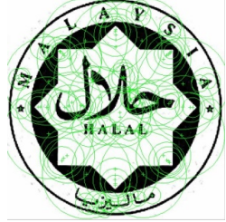
Fig-11: Detection of Interest Points in a Grayscale Image using SURF
