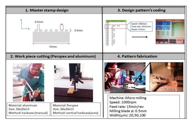
**Step 1** (machining): Micro-milling of Perspex material with optimized speed and feed rate. The difference between diced region is the technique to obtain micrometer dimension with milling edge of 0.5 mm.
