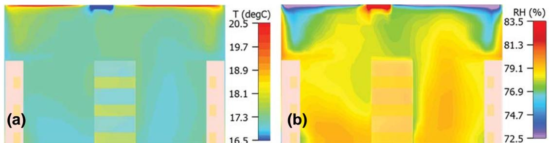
**Figure 6 – Thermohygric profile at  $x = 2.25\text{m}$  (a) T contour (b) RH contour**
