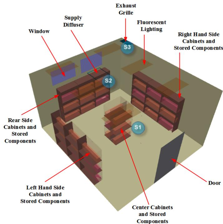
**Figure 2 – Space Layouts with positions of supply, exhaust and other components of the case study room. S1, S2 and S3 are virtual data loggers' positions**
