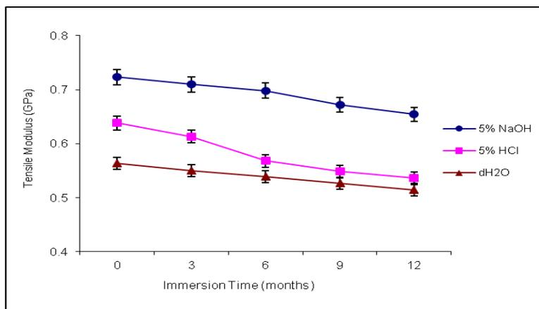
**Fig. 3.** Influence of the corrosion media on tensile modulus of vinyl ester composite filled with carbonized *Jatropha* seed shell. The tensile modulus for untreated composite was 0.715 GPa. Data presented as the mean  $\pm$  standard deviation.
