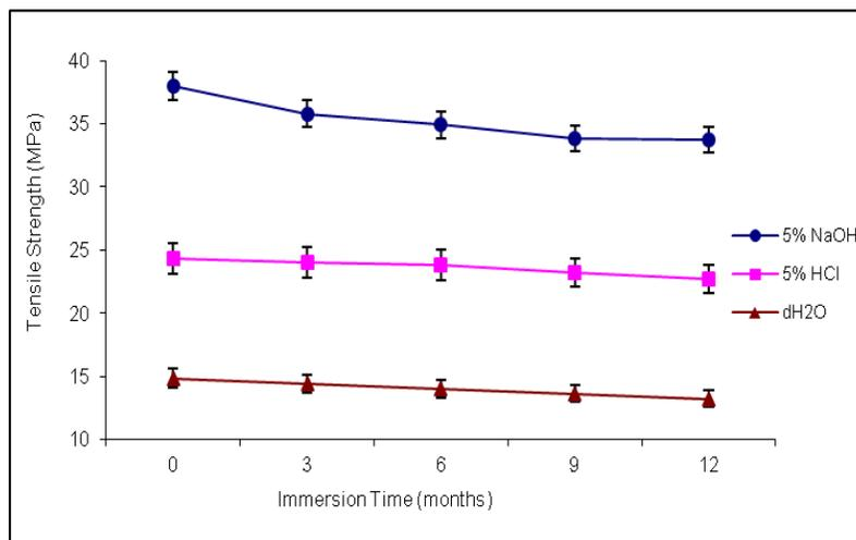
**Fig. 2.** Influence of the corrosion media on tensile strength of vinyl ester composite filled with carbonized *Jatropha* seed shell. The tensile strength of untreated composite panel was 44.92 MPa. Data presented as the mean  $\pm$  standard deviation.
