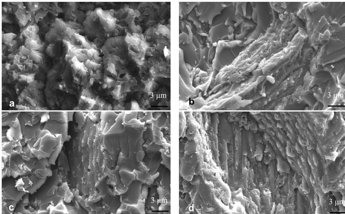
**Fig. 7.** SEM image of the carbon fiber of *Jatropha* seed shell filled vinyl ester composites: (a) Control (source: Sri Aprila *et al.* 2014) (b) after immersion in 5% NaOH for 12 months, (c) after immersion in 5% HCl for 12 months, and (d) after immersion in distilled water for 12 months
