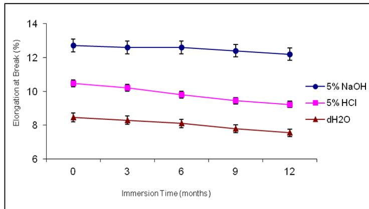
**Fig. 4.** Influence of the corrosion media on percentage loss in elongation at break of vinyl ester composite filled with carbonized *Jatropha* seed shell. The percentage elongation at break for untreated composite was 12.4%. Data presented as the mean  $\pm$  standard deviation.
