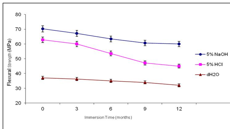
**Fig. 5.** Influences of the corrosion media on flexural strength of vinyl ester composite filled with carbonized *Jatropha* seed shell. Flexural strength of untreated composite panel, 119 MPa. Data presented as the mean  $\pm$  standard deviation.
