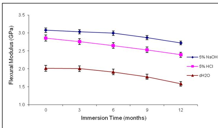
**Fig. 6.** Influence of the corrosion media on flexural modulus of vinyl ester composite filled with carbonized *Jatropha* seed. The flexural modulus for untreated composite was 2.91 GPa. Data presented as the mean  $\pm$  standard deviation.
