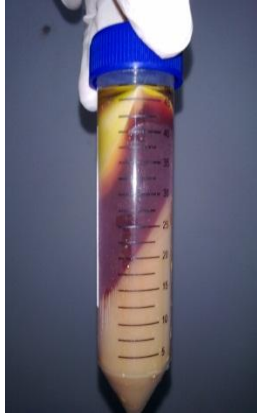
Figure 3: Mixture of viscera and buffer solution after centrifugation, the top layer is a layer of lipids, the second layer is the serum that is separated from the rest to be the crude enzyme and bottom layer is fine solids.
