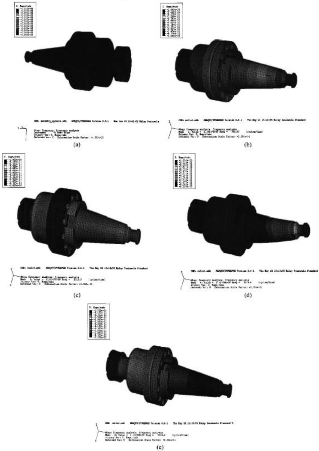
Figure 9 Selected eigenmodes of the collect by FE analysis, (a) base state (b) mode: 770.77 Hz (c) mode: 2,318.9 Hz (d) mode: 3,673.6 Hz (e) mode: 5,318.2 Hz (see online version for colours)
