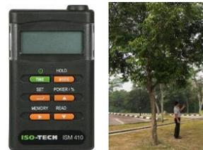
Fig. 4: The solar meter used and the process to measure solar radiation
