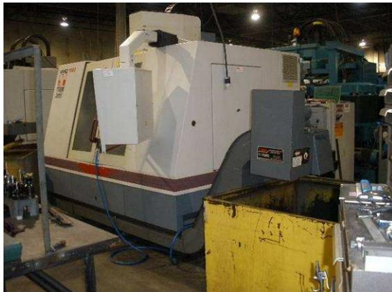
Fig. 1: VMC milling center
