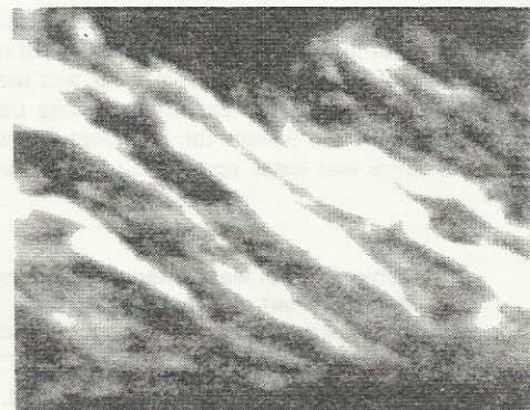
Fig. 15 Microstructure of chip after machining with preheating at 350°C for case I (Cutting condition: Cutting speed=100 m/min, depth of cut=1 mm and feed=0.1 mm per tooth)
