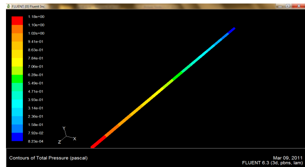
Fig.3: Contour of total pressure in boiler tube
