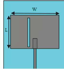
Figure 3. Patch antenna with one slot for 0.9 GHz
