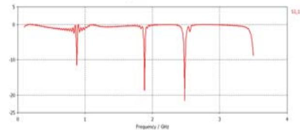
Figure 12. Plot of  $S_{11}$  (in dB) for an optimized antenna with resonant frequency at 0.9, 1.8 and 2.45 GHz.
