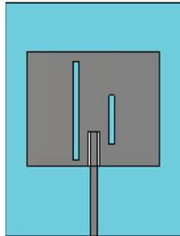
Figure 7. Patch antenna with slots for 0.9 and 1.8 GHz
