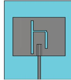
Figure 9. Patch antenna with slots for 0.9, 1.8 and 2.45 GHz
