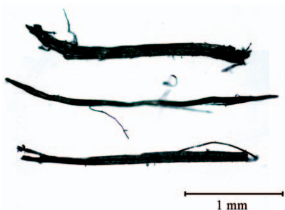
Figure 2. Optical micrograph of multifilament kenaf fiber observed under 5000 \times magnification.
