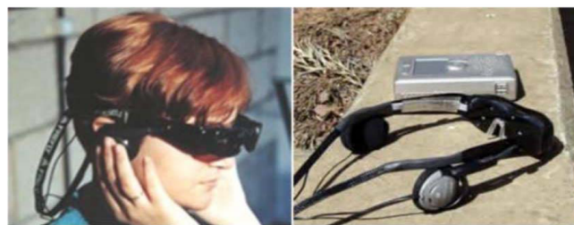
Figure 24 Virtual acoustic space prototypes (cameras and headphones mounted on eyeglasses and microprocessor) (right)
