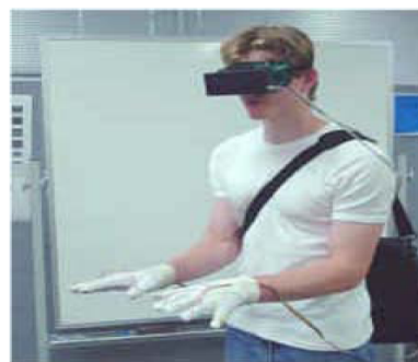
Figure 24 Virtual acoustic space prototypes (cameras and headphones mounted on eyeglasses and microprocessor) (right)
