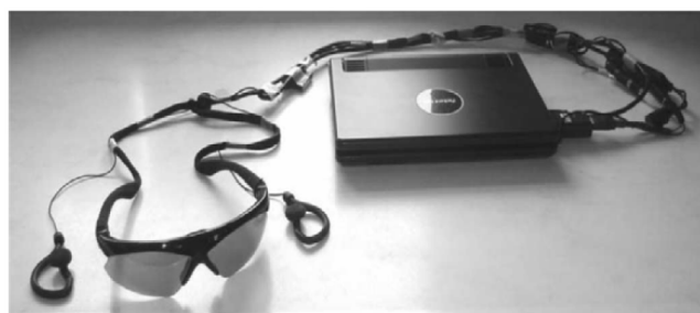
Figure 19 Implementation of the vOIce – 'seeing with sound' system
