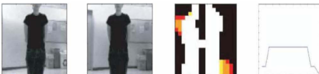
Figure 28 Example of TVS operation: image from the two cameras, disparity map, and the corresponding signals sent to the tactile belt
