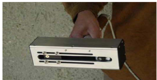
Figure 29 UCSC's handheld device equipped with laser range sensor
