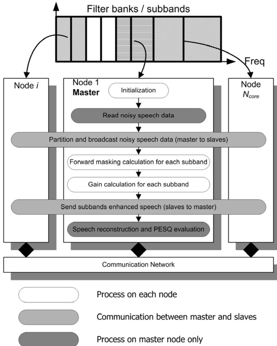
Fig. 4: Flowchart of parallel speech enhancement algorithm.
