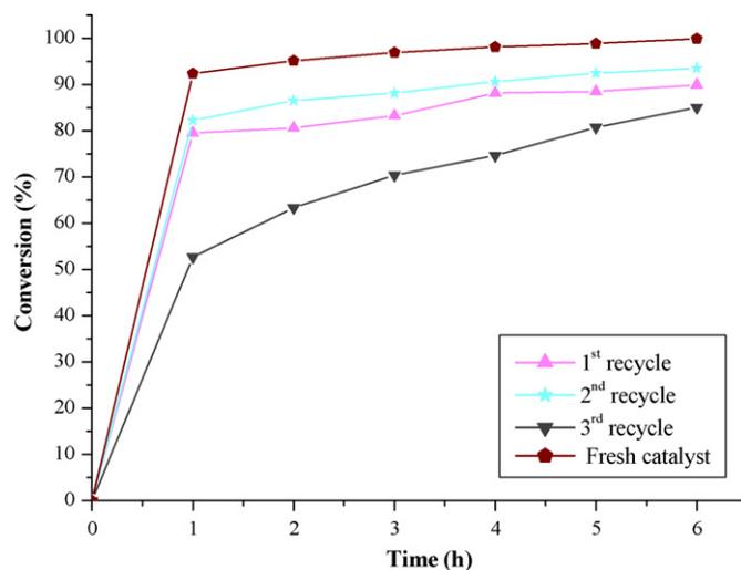
**Fig. 12.** The graph of percentage conversion of styrene with recycled RHCr-3 showing small loss in conversion. The mass of catalyst used was 100 mg. Reaction temperature was 353 K and 1:4 molar ratio of reactants.
