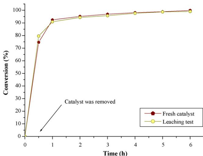
**Fig. 11.** The graph of percentage conversion of styrene during leaching test using fresh RHCr-3. The mass of catalyst used was 100 mg. Reaction temperature was 353 K and 1:4 molar ratio of reactants. The catalyst was removed after 30 min and the reaction allowed to continue to completion in 6 h.
