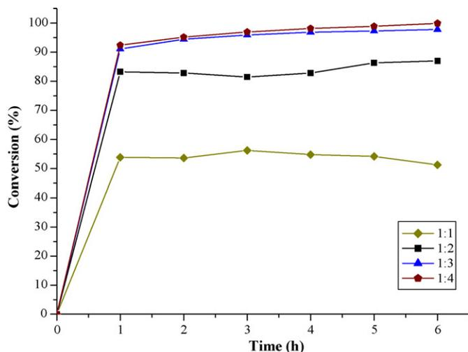
**Fig. 8.** The effect of reactant molar ratio on the percentage conversion during oxidation of styrene by  $\text{H}_2\text{O}_2$ . 100 mg of RHCr-3 was used and the reaction temperature was 353 K.
