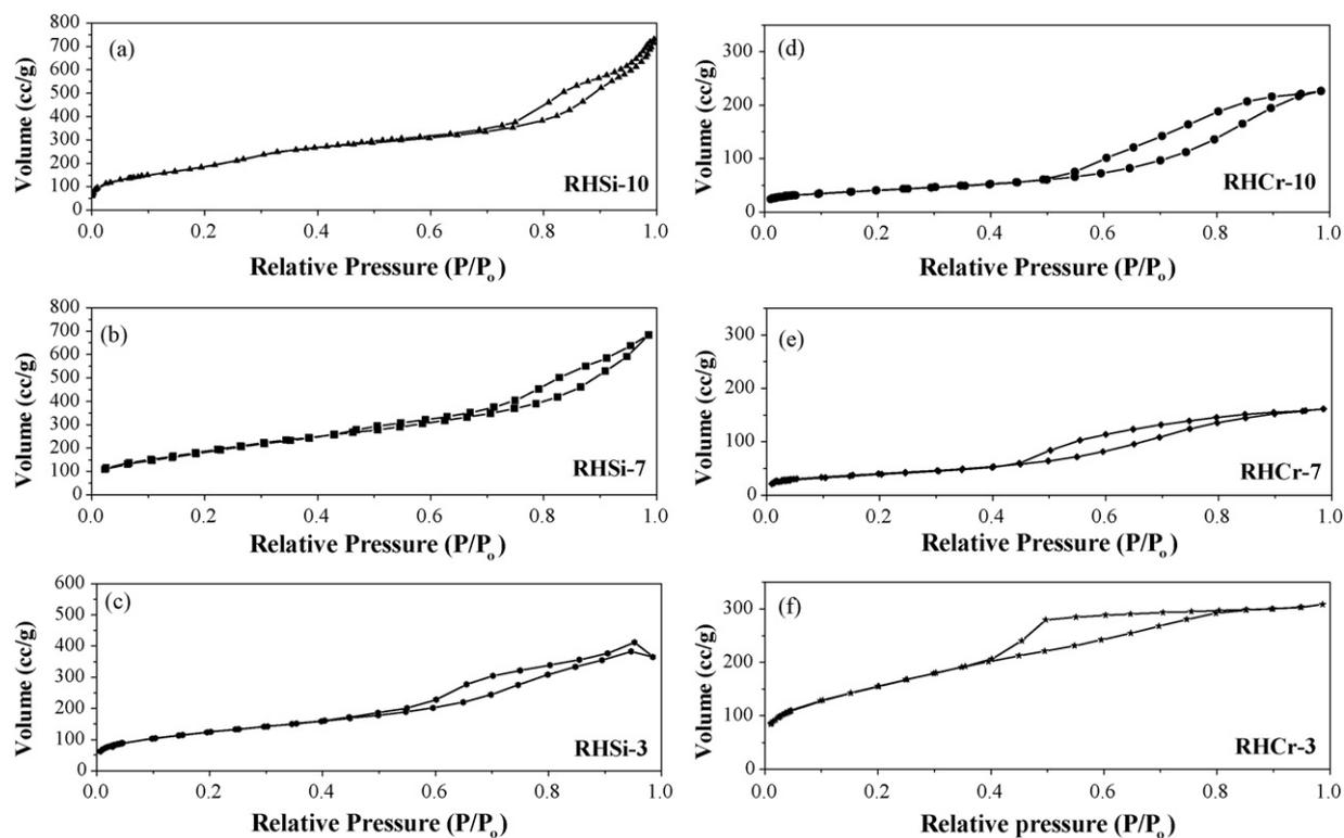
Fig. 2. The nitrogen sorption isotherm of (a) RHSi-10, (b) RHSi-7, (c) RHSi-3, (d) RHCr-10, (e) RHCr-7 and (f) RHCr-3.
