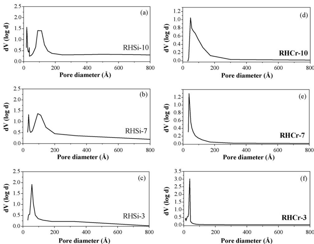
Fig. 3. Pore size distribution for (a) RHSi-10, (b) RHSi-7, (c) RHSi-3, (d) RHCr-10, (e) RHCr-7 and (f) RHCr-3.
