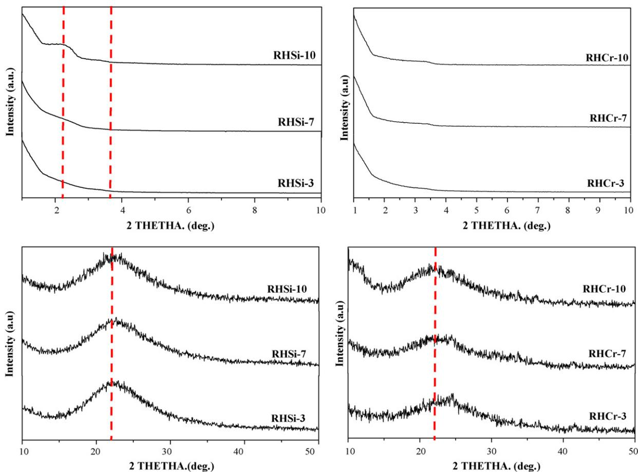
Fig. 1. The low and high angle X-ray diffraction pattern for the prepared catalyst.
