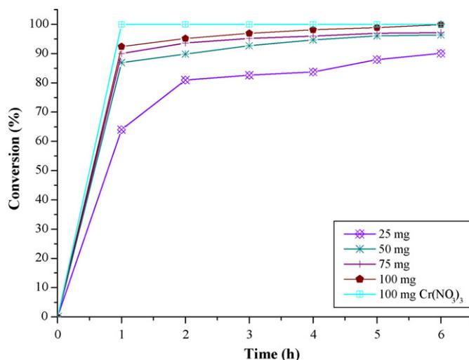
**Fig. 10.** The percentage conversion of styrene oxidation with different masses of RHCr-3 as the catalyst. 1:4 styrene to  $\text{H}_2\text{O}_2$  was used and the reaction was carried out at 353 K. The catalytic activity of the homogeneous salt  $[\text{Cr}(\text{NO}_3)_3 \cdot 9\text{H}_2\text{O}]$ , 100 mg has been included for comparison.
