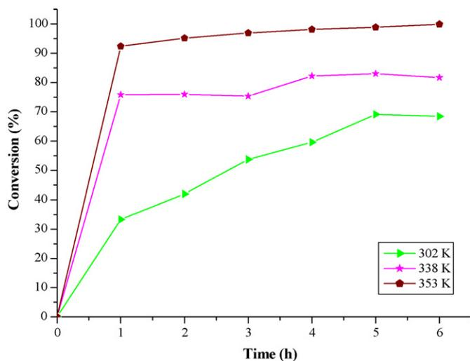
**Fig. 9.** The effect of reaction temperature on the percentage conversion of styrene. The mass of RHCr-3 used was 100 mg with a 1:4 molar ratio of reactants.
