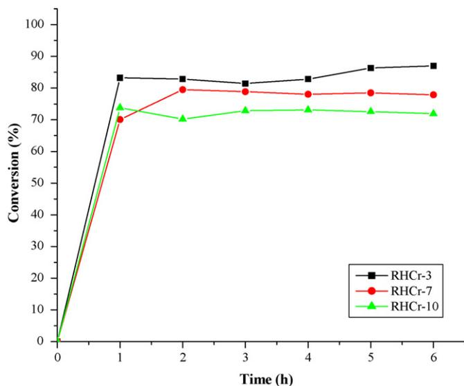
**Fig. 7.** The effect of preparation pH of catalyst on the percentage conversion during oxidation of styrene by  $\text{H}_2\text{O}_2$ . 100 mg of catalyst was used with 1:2 styrene to  $\text{H}_2\text{O}_2$  molar ratio. The reaction was carried out at 353 K.
