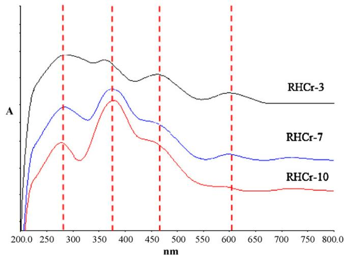
Fig. 4. The UV–vis diffuse reflectance spectra of RHCr-10, RHCr-7 and RHCr-3.
