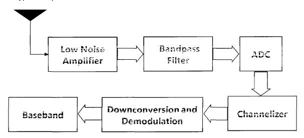
Figure 21.3: Architecture of a Generic Software Radio
