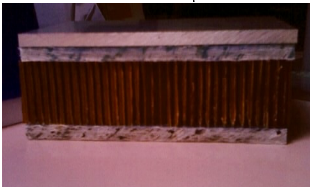
Figure 11 Multi-wall construction of fuel tank.
