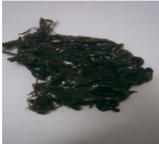
Figure 2: Biocomposite (PLA+Kenaf+Plasticizer) at 180 0 C which indicates the burning of fiber.
