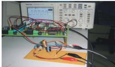
**Fig. 13:** Testing the buck converter.
