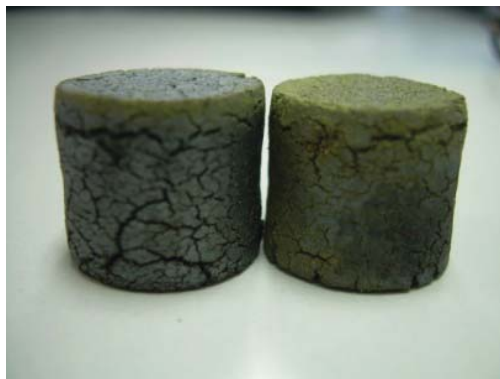
Fig. 4 Electrodes sintered at 850 °C for 50 min.
