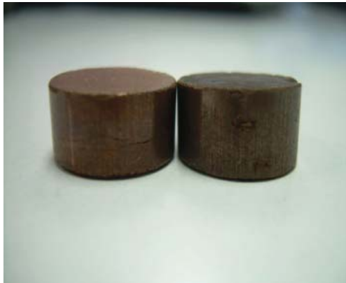
Fig. 2 Green compacted electrodes.
