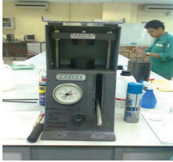
Fig. 1 The carver press used for compaction.
