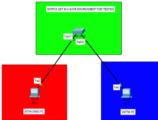
Fig. 1. Setting up of network topology for experimental testbed for dataset collection.
