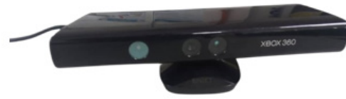
FIGURE 2. XBOX 360 model RGB-D (Micro Kinect) Camera
