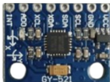
FIGURE 6. IMU Sensor used in wrist attachment
