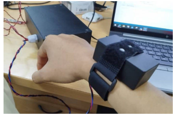
FIGURE 4. IMU sensor mimics wristwatch for measuring arm movement.
