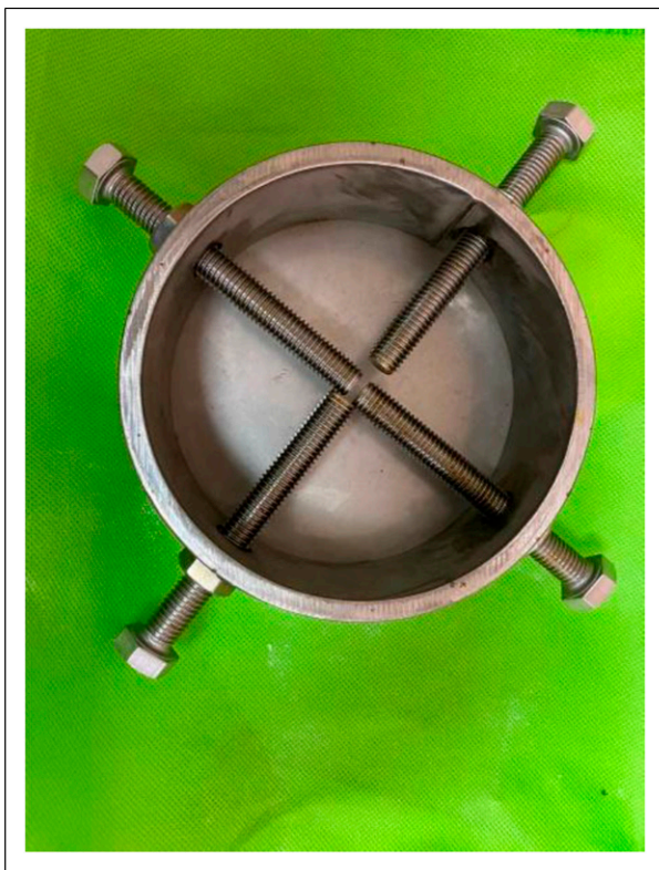
Figure 3. The tibia clamp used to secure the synthetic tibia bone model.
