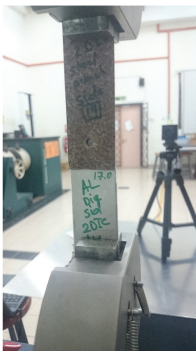
Figure 3. Universal shear tension machine with clinching sample.
