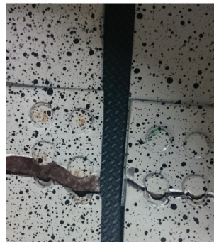
Figure 4. Clinching joints with different configurations with white and black pattern and failure modes.
