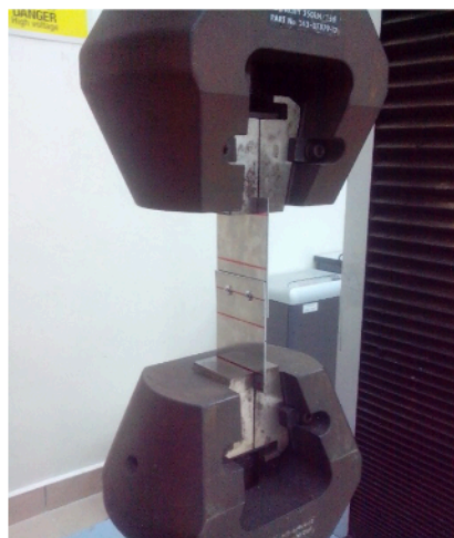
Fig. 4. Tensile shear testing setup
