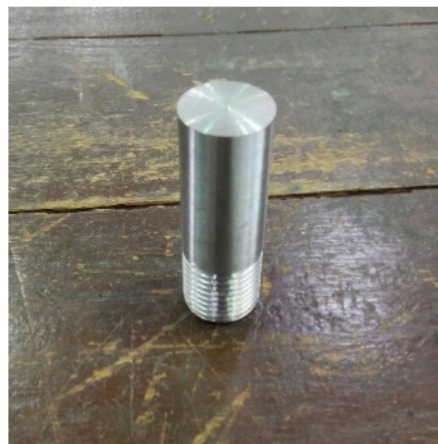
Fig. 5. Flat die for reshaping process
