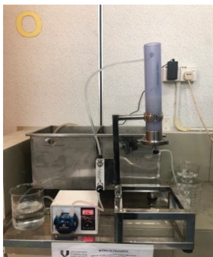
Figure 3. The experimental setup for packed-bed filter (dimension: 20 cm length, 4.3 cm inner diameter)
