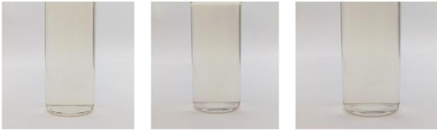
**Fig. 2.** The optimised formulation showing no turbidity and good stability after centrifugation at 5000 rpm for 30 min, three consecutive heating-cooling cycles (40 °C and 4 °C) for 24 h, and a freeze-thaw cycle for 24 h (-5 °C and 25 °C). Formulation was tested in triplicates.
